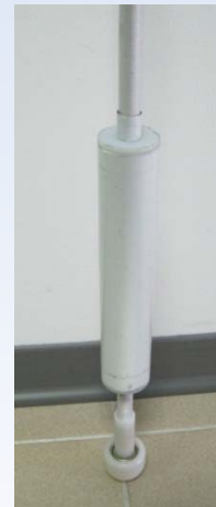
The path detector fitting inside an ad-hoc developed fiberglass case
